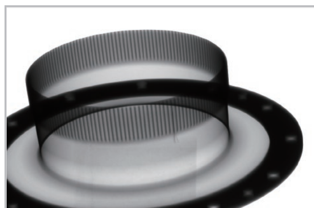
柔轮无损探伤检测 Nondestructive testing for FS
